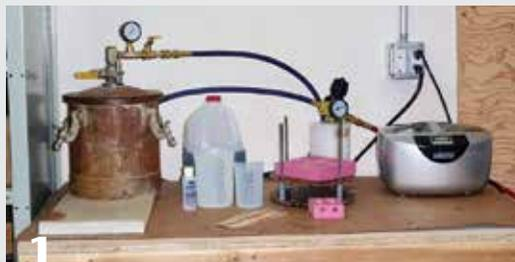
Some useful but optional pen-casting items include a pressure pot, air compressor, ultrasonic cleaner, and a warming oven. At a minimum, you'll need the resin and catalyst, as well as a mold.
