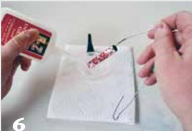
After the white glue has dried thoroughly, apply thin CA glue to seal the paper. This is necessary because paper is porous and could release air bubbles into the resin during casting.
