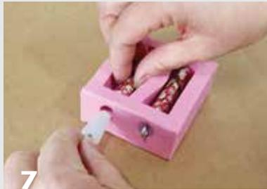
After the CA glue has cured, set the blanks into the mold in preparation for pouring. A silicone mold has separate compartments for each pen tube. End plugs center and suspend the tubes so the resin can flow all the way around them.
